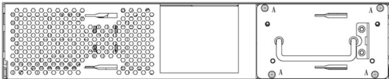
Note: Remove four M4\*6 screws marked with letter A on the disassembly figure.
